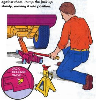
RATCHET the jack stand's saddles up into place, and then lower the service jack until the jack stands are supporting the vehicle. Never put any additional saddles on top of either the service jack or the jack stands, as they can slip off—and you wouldn't want to be underneath when it happens!
