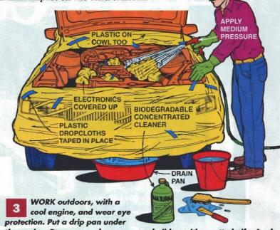
the engine. Remove any heavy grease buildup with a putty knife. Apply the cleaner according to instructions, and wash it off using medium water pressure. Use as little water as possible, rinsing from the top down. Don't use a pressure washer and don't spray water directly onto any electrical wires, oil fill caps or dipsticks. Then remove the plastic covers from the engine components (but not the cowl or fenders), start the engine, and let
