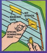
APPLY the special paint carefully and smoothly, overlapping it onto the original paint. Once completely dry, remove the stencil or masking tape. Carefully trim any excess paint with the razor blade.
