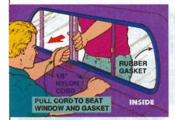
OPEN the sliding glass and push the window and gasket into place on your pickup, from the outside. Make sure you've got the cord ends inside. Have a helper hold the window in place while you slowly pull the cord toward the dashboard, seating the gasket. Pull the cord from the bottom and work both ways equally. Make sure the gasket is tight along the inside of the cab. Wash the window and you're ready to go out and catch a breeze.
