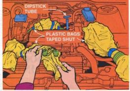
components with plastic bags secured with tape and rubber bands. Put plastic dropcloths on the cowl and both fenders to protect the paint against spotting and overspray.
