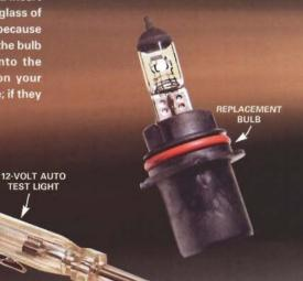
Test for power at the socket. Turn on the light switch, then ground the tester to a clean screw on the body of the car. Probe the contacts to see if the tester lights. If the contacts look corroded, scratch the surface, but be careful not to bend or distort them. The tester should light for two out of three contacts (one won't because it's a ground). If two of them light, insert the bulb. If the bulb still only one or no contact shows power. go to Step 4.
