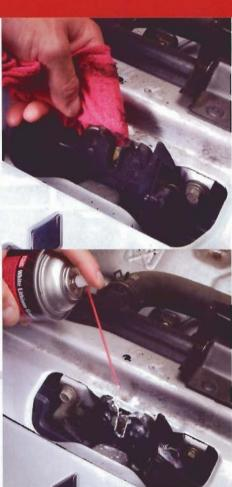
Hood latch 5 Wipe the grime and dirt away with a clean cloth. Try to get any bits of sand that may be embedded in the existing grease. If you see rusted or stuck parts, give the latch a spray of WD-40, then move the mechanism several times. Wipe it again and give it a liberal coating of white lithium grease.
