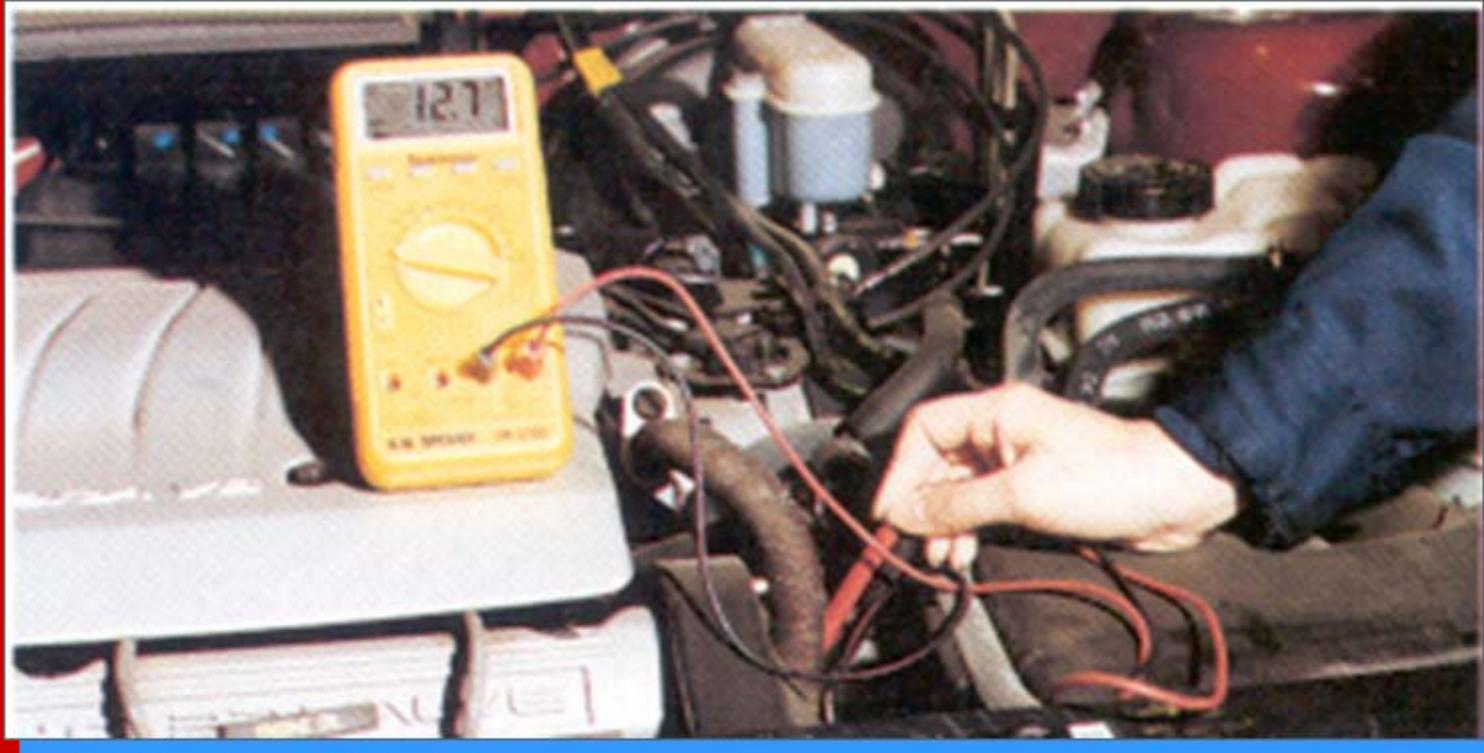
Also called a DVOM—combines an ohmmeter, ammeter, and voltmeter in one tool
