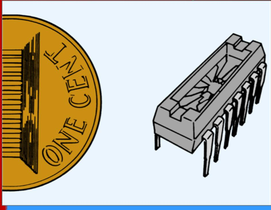
Contains microscopic diodes, transistors, resistors, and capacitors in a wafer-like chip
