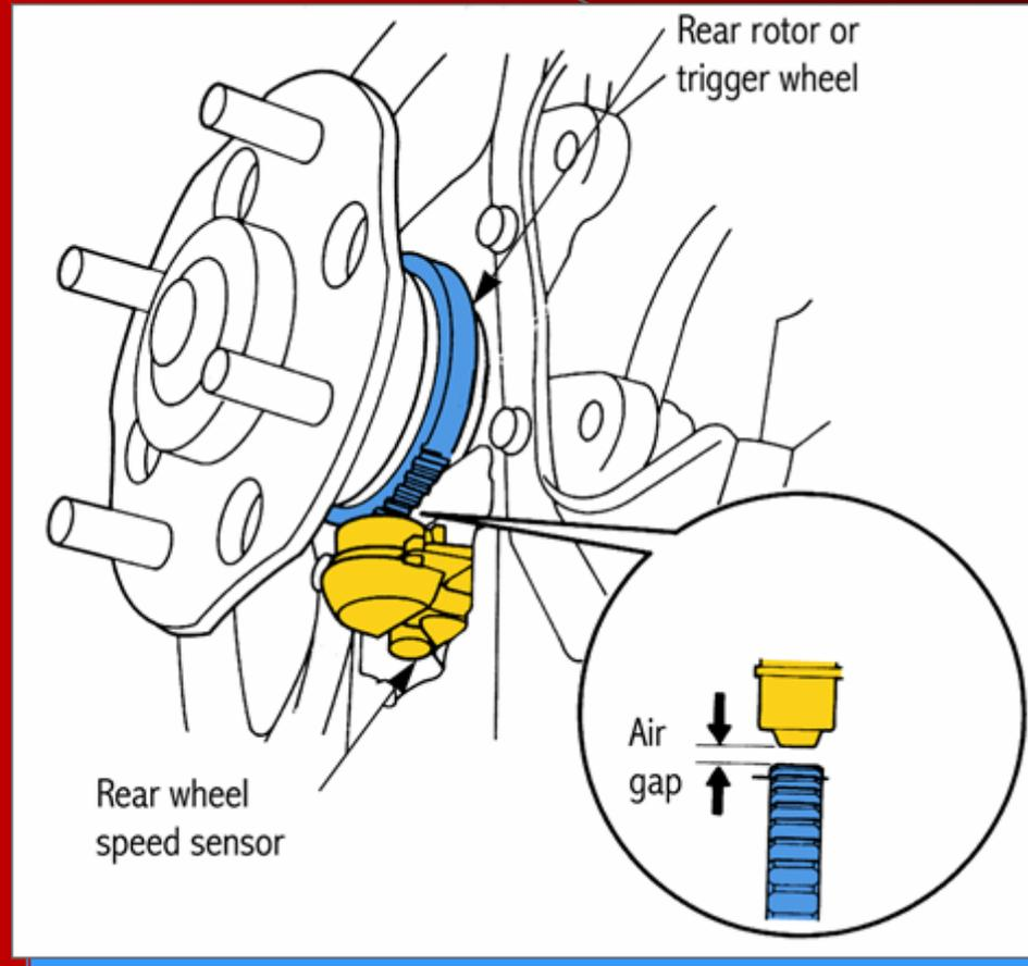
If applicable, use a non-magnetic (brass) feeler gauge to check the air gap
