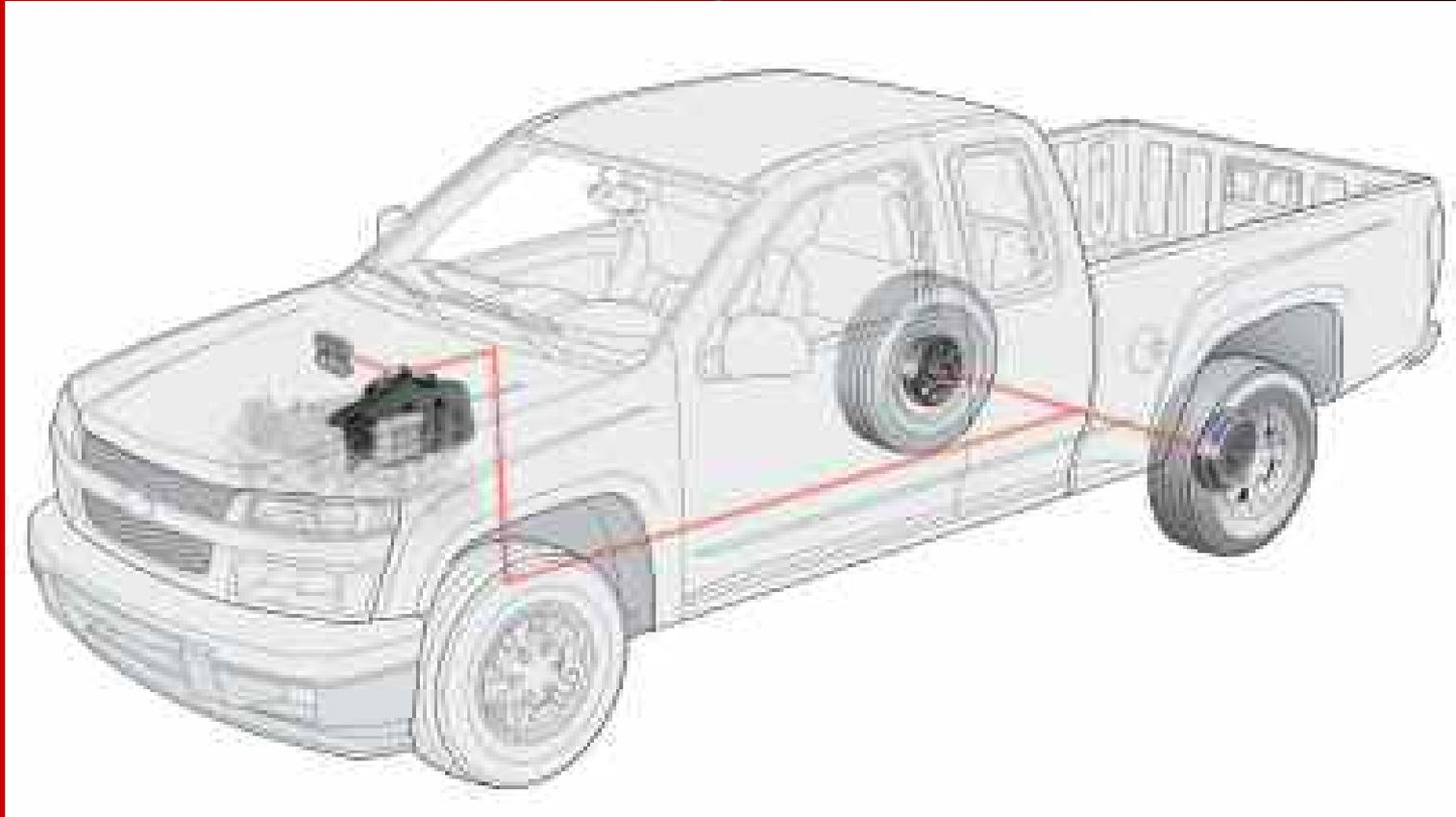
Traction control systems use the ABS system to limit power to the drive wheels to prevent wheel spin under acceleration.
