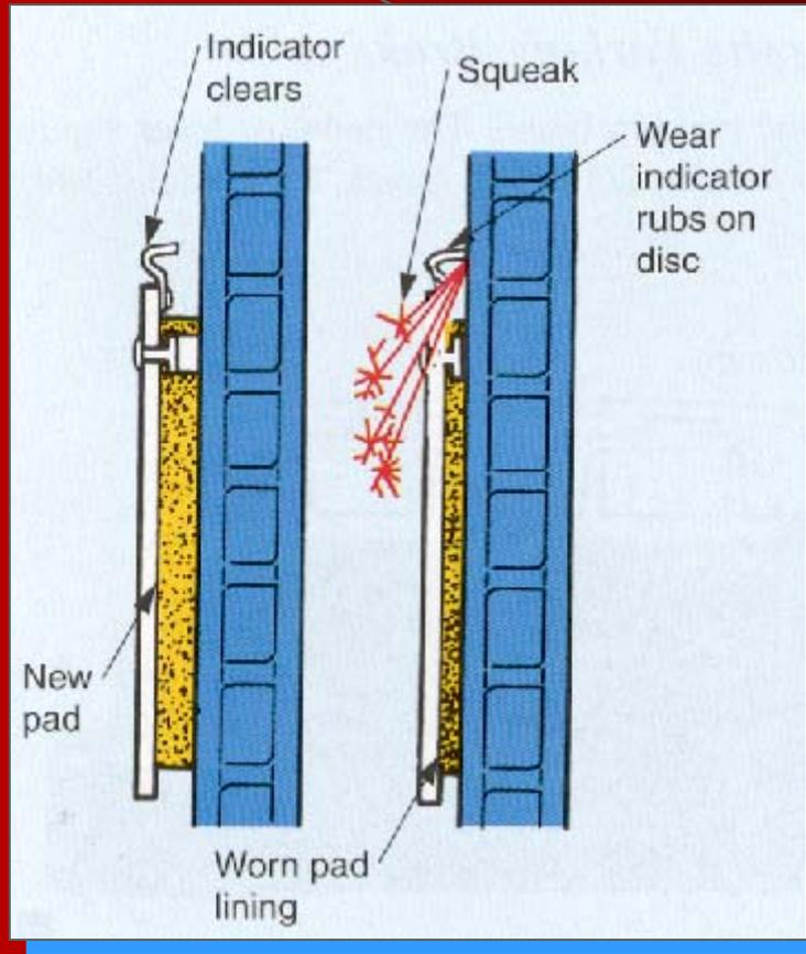
Inspect brake pad linings for thickness, must not be less than  $1/16''$  ( $2/32''$ , 1.5 mm).
