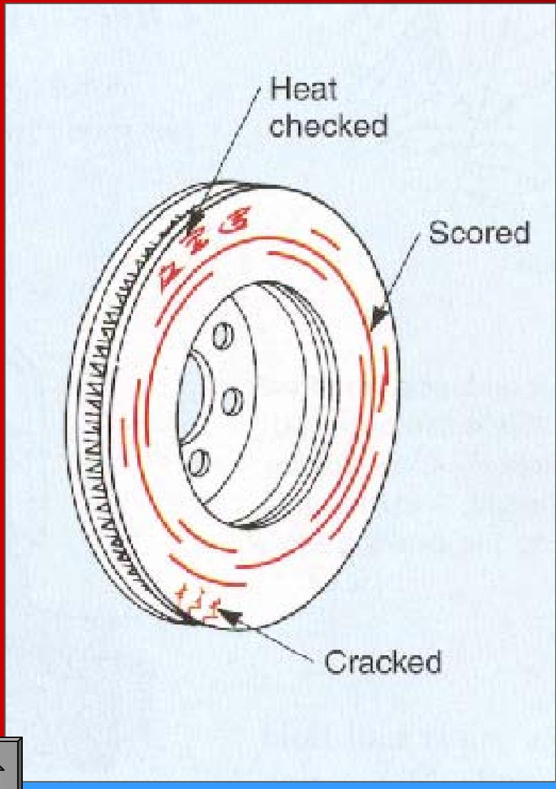
Inspect rotors: scoring, cracks, out-of-round, and/or heat damage can cause brake pedal vibration
