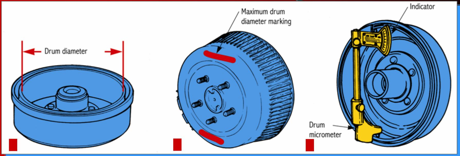
Typically, a drum should not be machined more than 0.060" (1.5 mm) oversize
