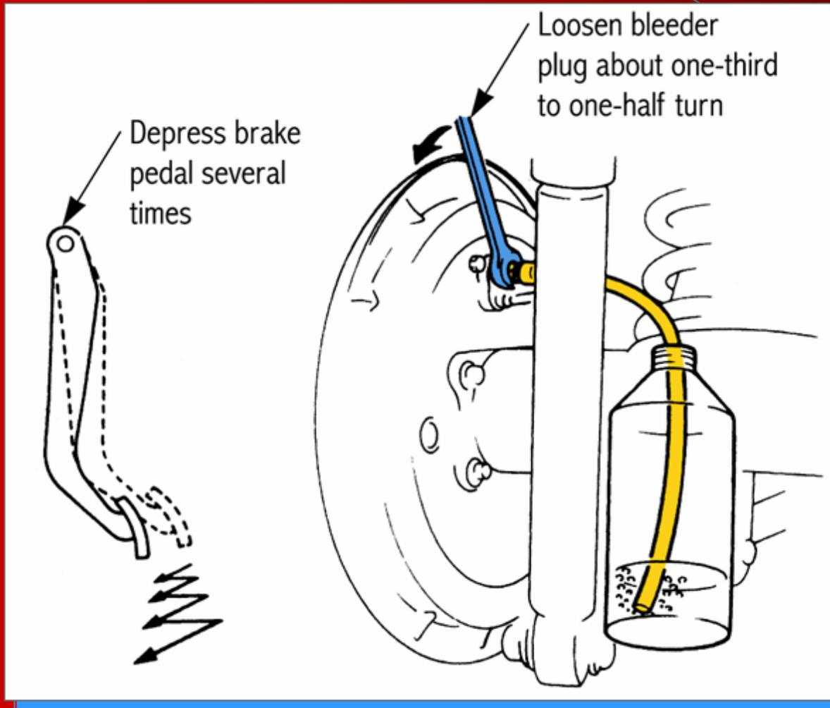
Bleeding brakes removes air from the brake system
