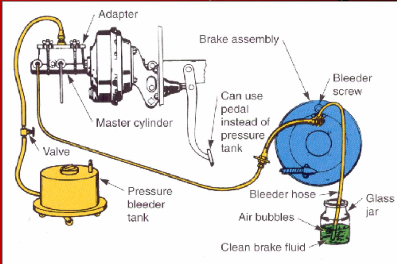
Uses a pressure bleeder tank, which contains brake fluid under pressure
