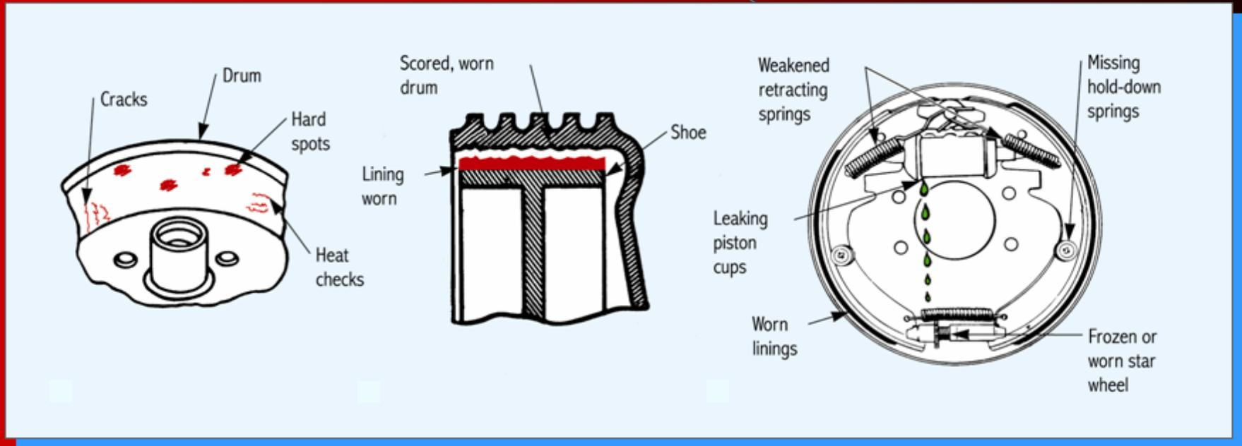
Check the drum for cracks or heat damage
