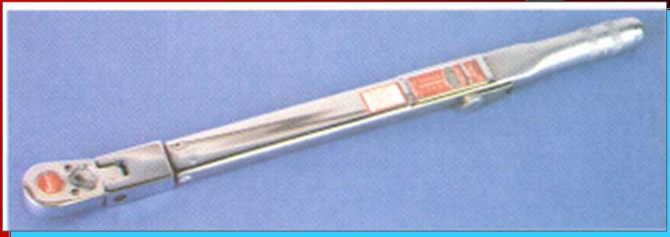
Torque value is set by turning the handle—
