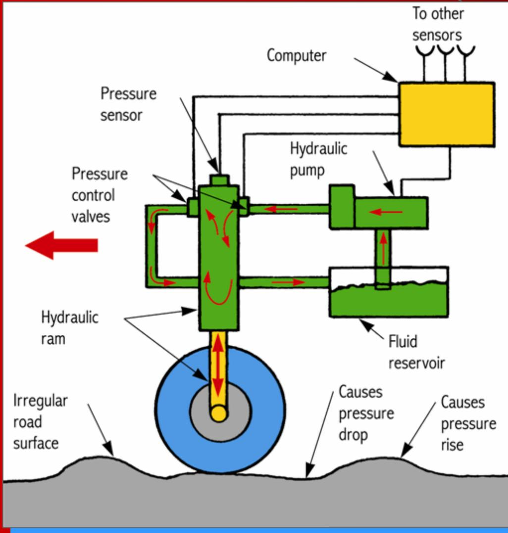
An Active Suspension System uses a hydraulic pump provides pressure to operate the rams
