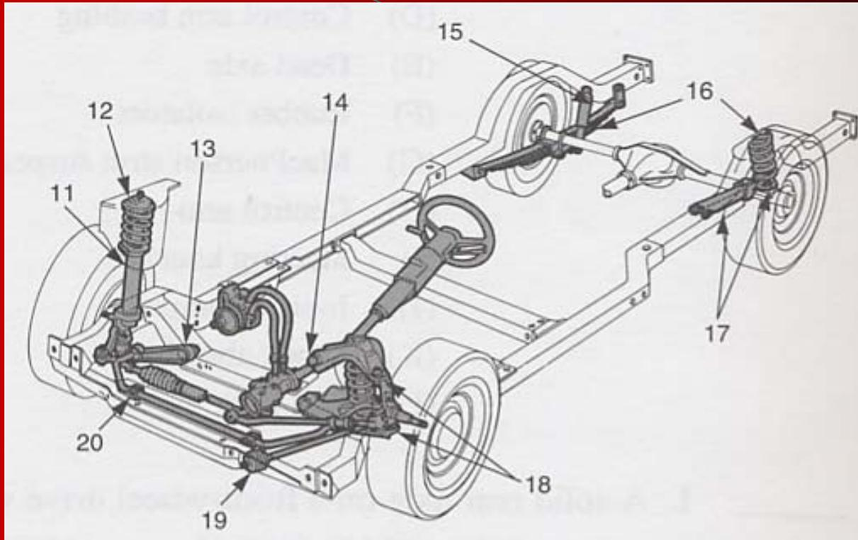
11. Bad strut shock 12. Worn upper strut mount 13. Bad control arm bushings 14. Worn upper control arm bushings 15. Bad shock absorber 16. Weak springs 17. Worn rear control arm bushings 18. Bad ball joints 19. Strut rod bushings worn 20. Sway arm bushings loose
