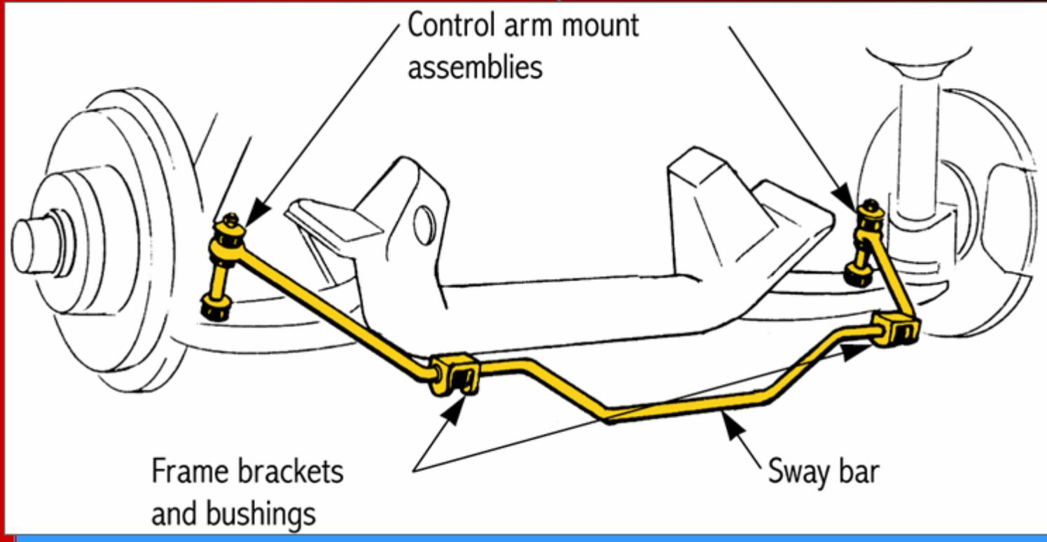
The sway bar links connect the Sway bar to the control arms
