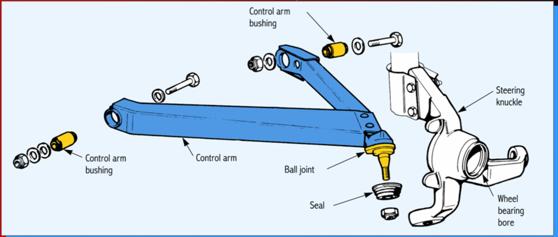
The separate parts that make up the control arm assembly.
