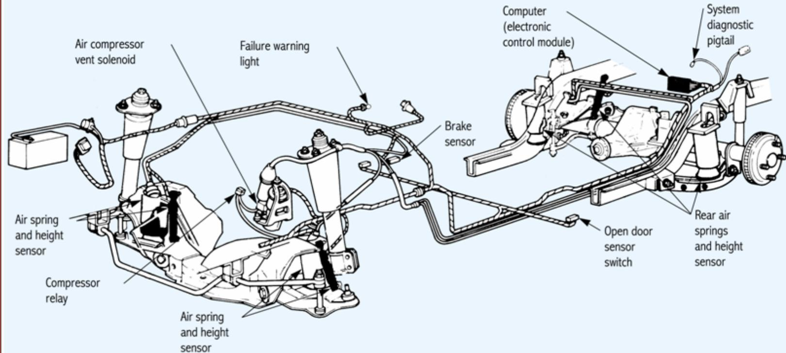
An Electric Height Control system uses height sensors and an electronic control module to control the operation of a small electric air compressor, which maintains the correct ride height
