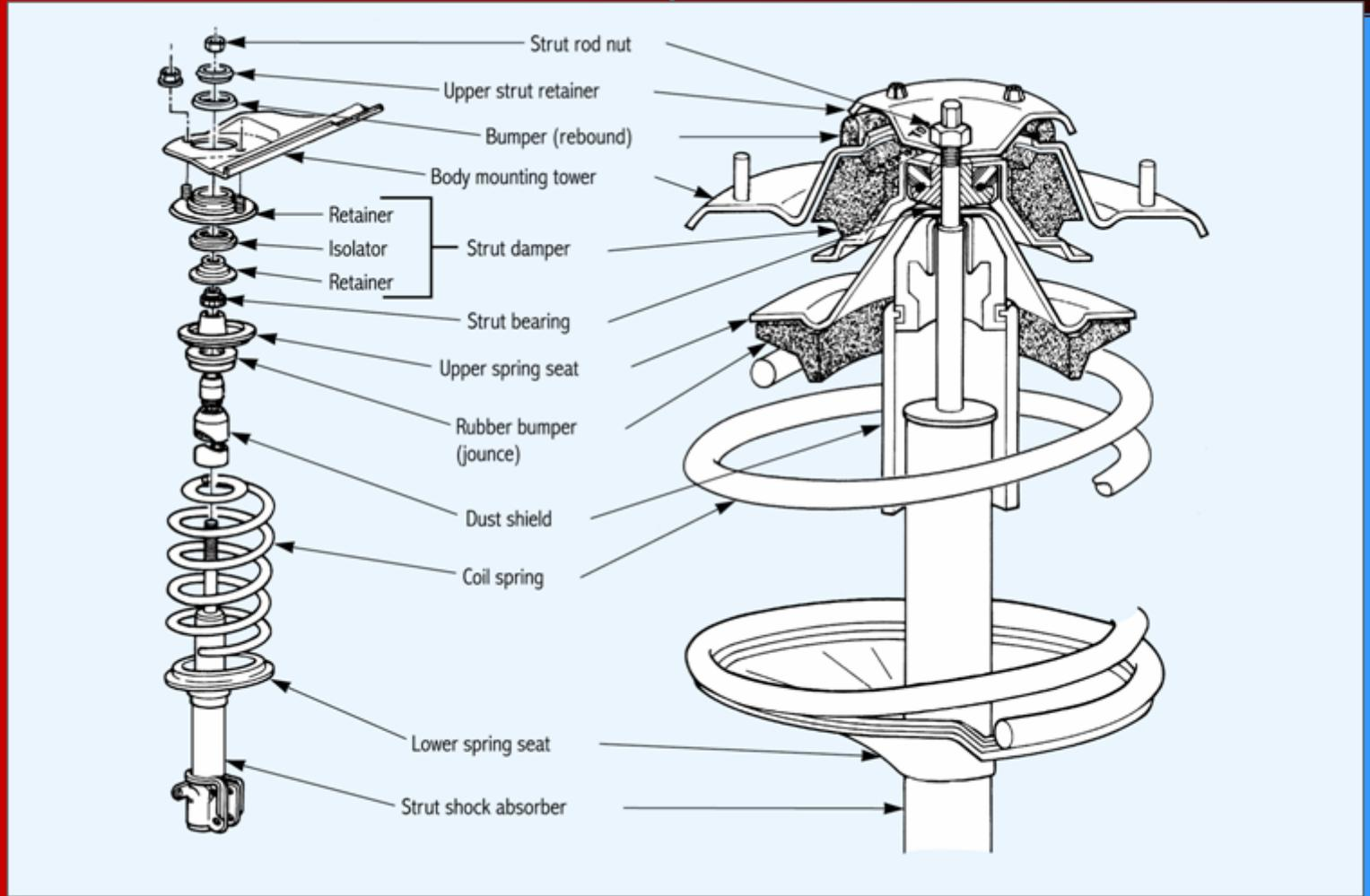
Parts of a MacPherson Strut Assembly
