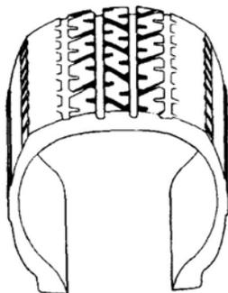
**C-Underinflation.** When a tire is underinflated, most of its contact with road is on outer tread rib, or shoulder, causing faster wear here than in middle. Be sure to check tire's air pressure.
