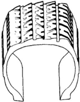
**A-Feathering.** This is caused by erratic scrubbing against road when tire is in need of toe-in or toe-out alignment correction.
