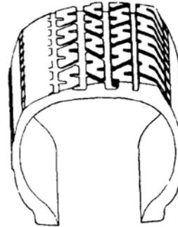
**D-One-side wear.** Here's another type of alignment problem—excessive camber, which means tire is leaning too much to inside or outside of tread, and placing all work on one side of tire.
