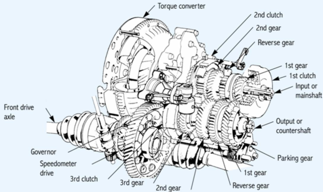
No planetary gear set is used
