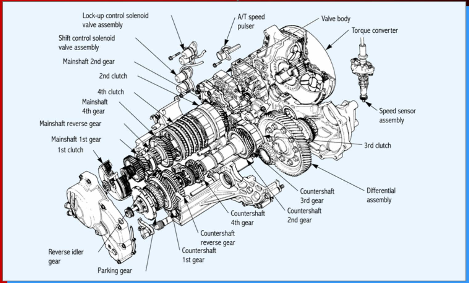
Solenoids and clutches control helical gears and torque converter lockup
