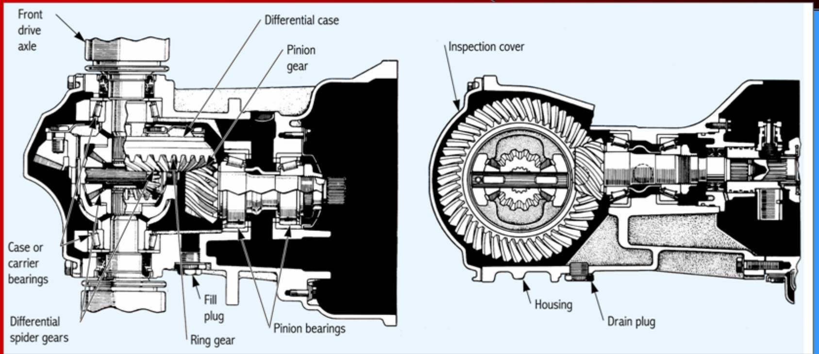
Hypoid gears transfer driving power
