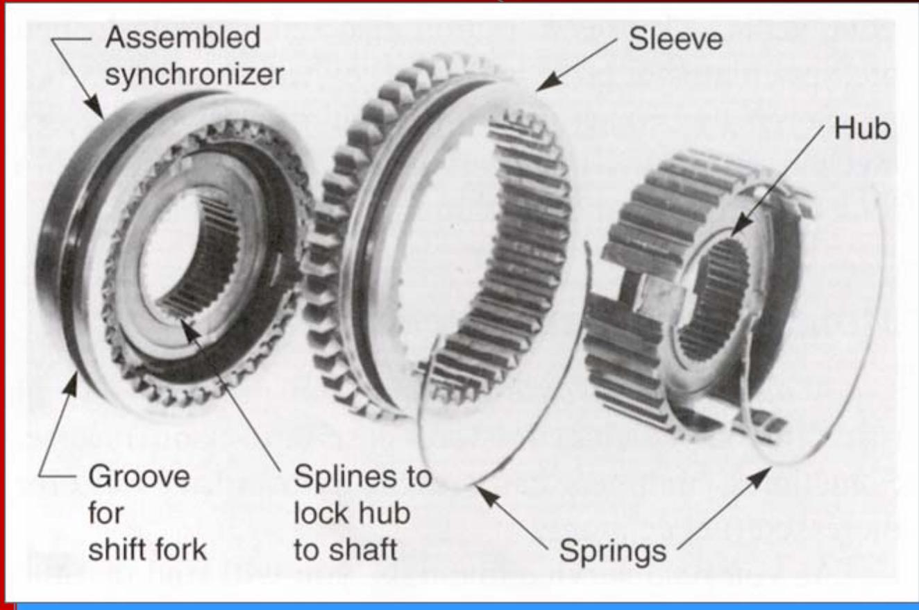
Inner hub is splined to a transaxle shaft. Outer sleeve is free to slide on the hub
