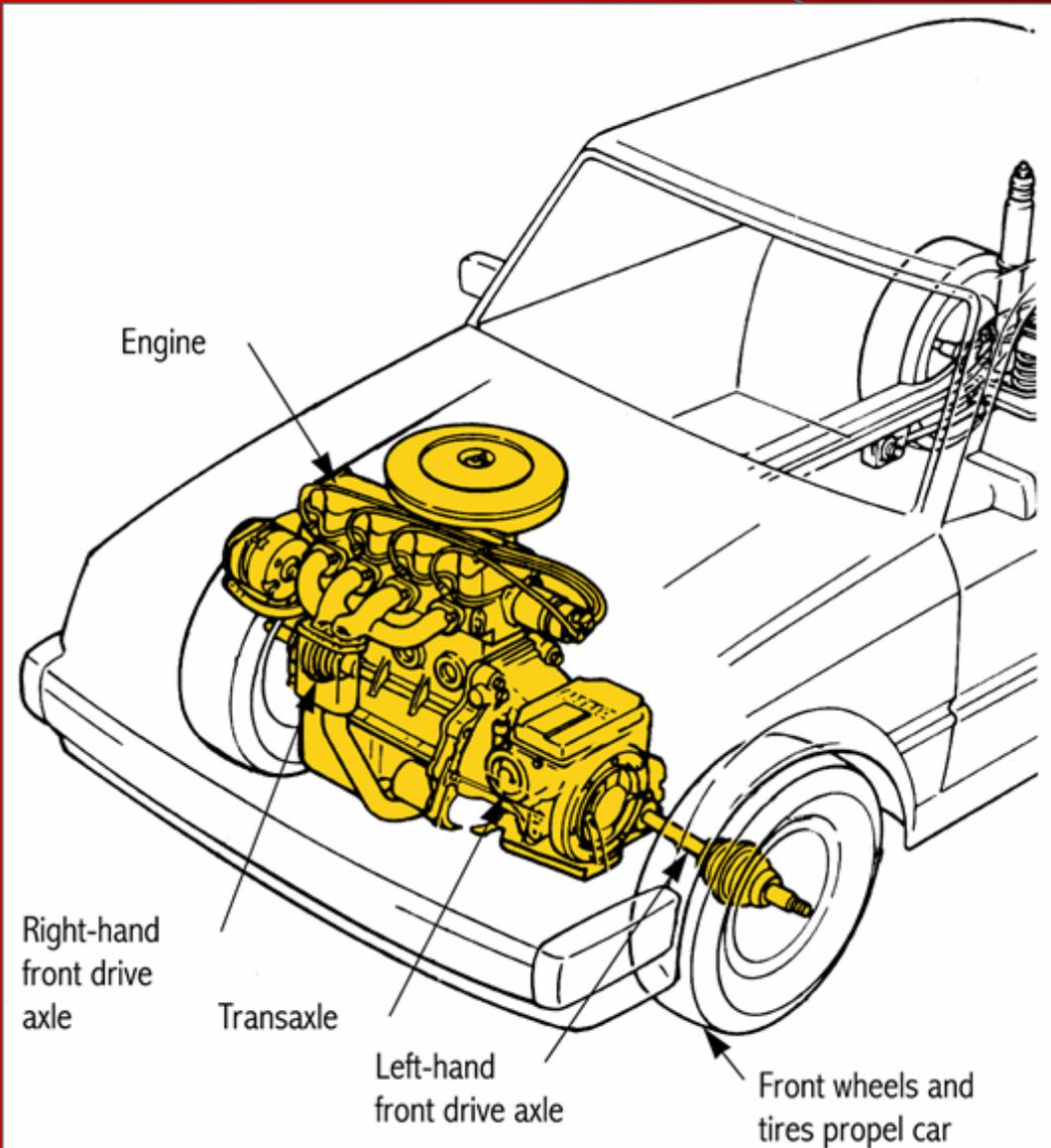
Short drive axle assemblies connect the transaxle output to the hubs and wheels
