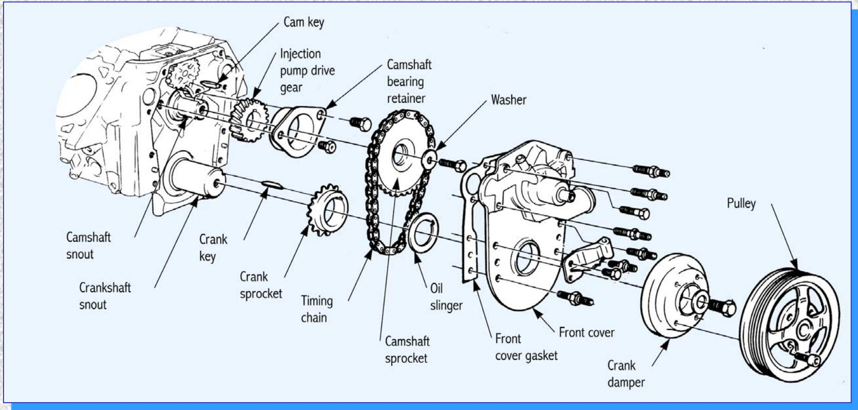
V-type, diesel engine with timing chain
