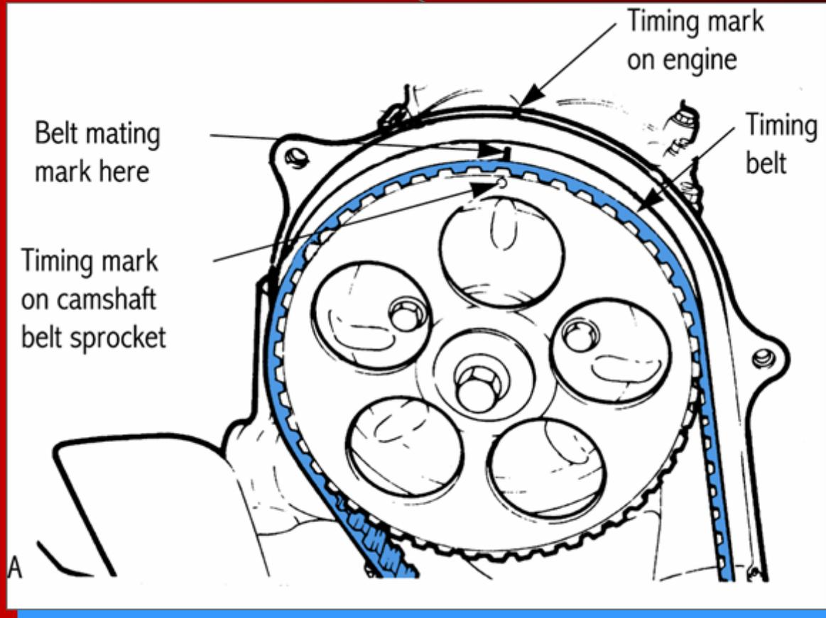
The camshaft sprocket mark is aligned with the belt marking and the timing mark on the engine
