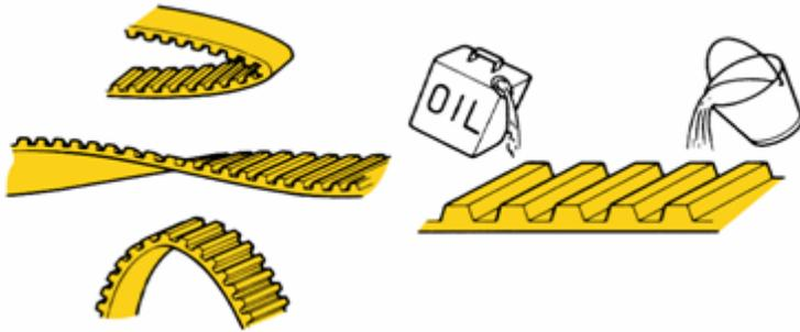
A—Do not bend, twist, or turn belt excessively. Oil and water will deteriorate belt. Fix all engine leaks.
