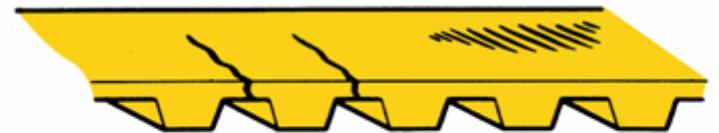
D—If there is wear or cracks on smooth side of belt, check idler or tensioner pulley.
