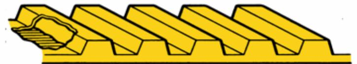
F—Wear on timing belt teeth may be caused by timing sprocket problem. Inspect sprockets carefully. Oil contamination will also cause this trouble.
