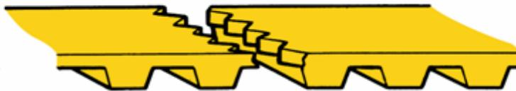
B—Belt breakage may be caused by sprocket or tensioner problem. Check these parts before installing new belt.
