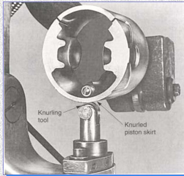
Increases skirt diameter by squeezing metal outward around small dents
