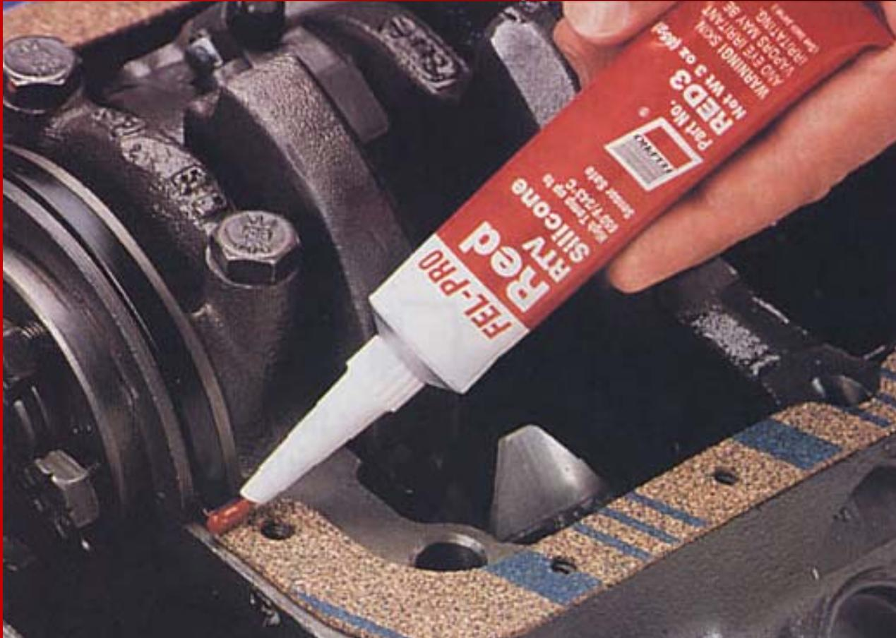
Installing RTV where the gasket meets a rubber seal. This is to prevent leakage
