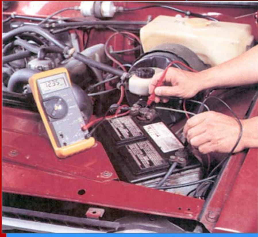
This technician is using a digital voltmeter to measure battery voltage
