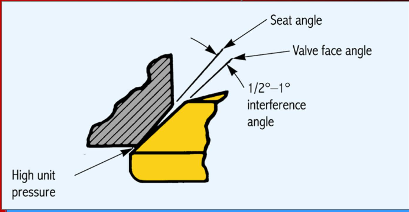
Interference angle increases sealing pressure and speeds seating
