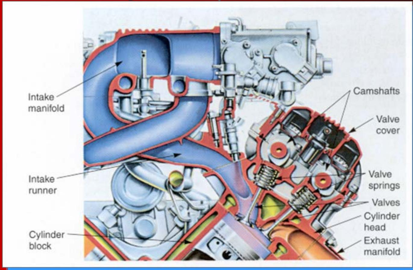
Includes the cylinder head, valve train, valve cover, and intake and exhaust manifolds
