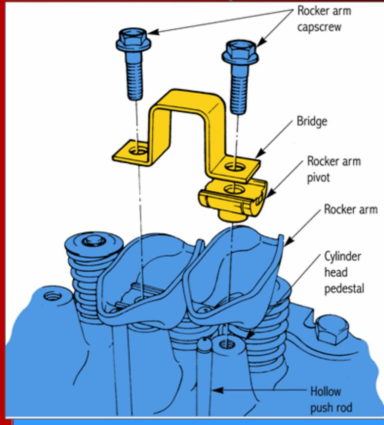
Used to hold the rocker arm in place over the valve
