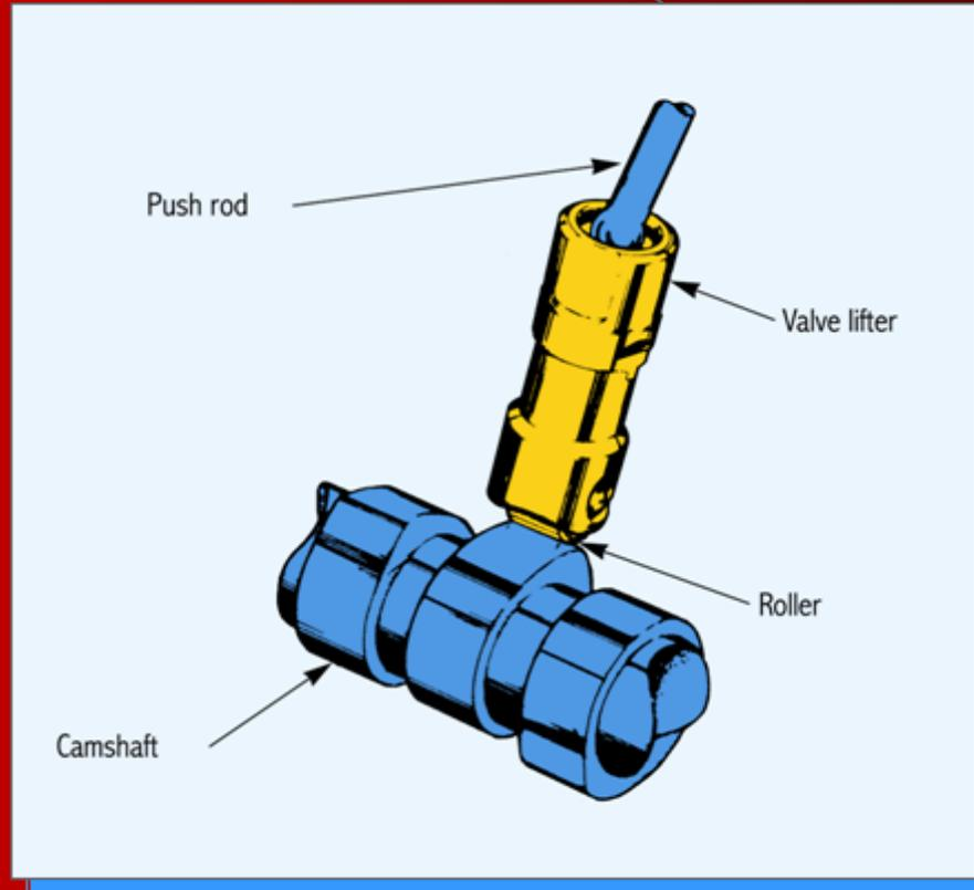
Small roller rides on the camshaft lobe to reduce friction
