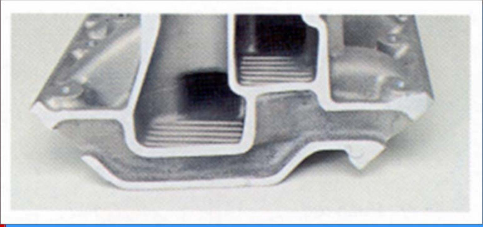
Carry either the air-fuel mixture or air to the cylinder head ports
