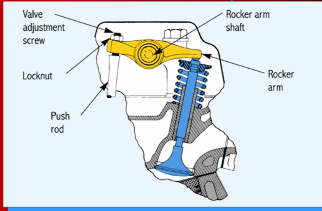
Transfer valve train motion to the valve stem tips
