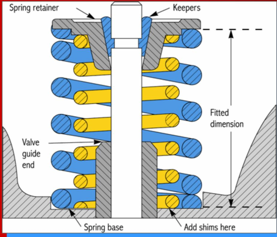
Very thin, accurately machined washer used to increase spring tension
