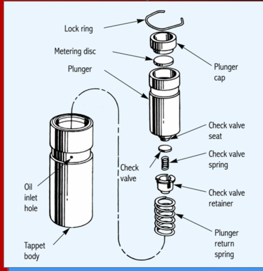
Lifter adjusts automatically with temperature changes and part wear
